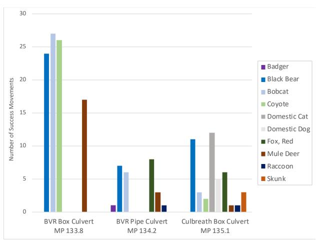
*Figure 20.* Success movements by species at each of the small culverts. Total monitoring days at each location are: BVR Box Culvert – 408 days; BVR Pipe Culvert – 306 days; Culbreath Box Culvert – 474 days.
