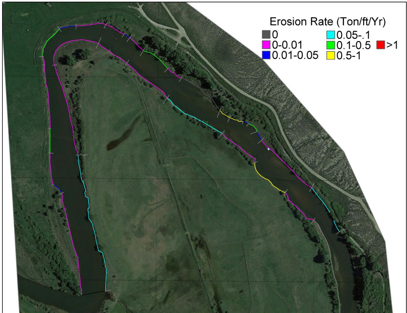
Figure 1. Streambank erosion rates in tons/yr/ft by location.
